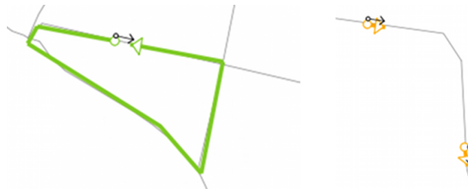
Figure 7: left: correctly modelled one-way street; right: missing one-way restriction. (narrow black arrows: extracted section against the one-way direction; wide colored arrows: routes generated on the comparison graph)
