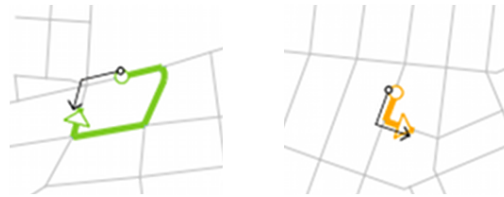
Figure 5: left: correctly modelled turn restriction; right: missing restriction on the right. (narrow black arrows: forbidden turn maneuvers; colored arrows: routes generated by routing on the comparison graph)
